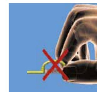
Never push inside the strip into the head like the two picture above. because you will not have enough force, and you risk to break the shank /blade of the strip.
