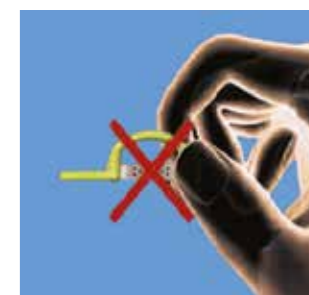
Never push inside the strip into the head like the two picture above. because you will not have enough force, and you risk to break the shank /blade of the strip.
